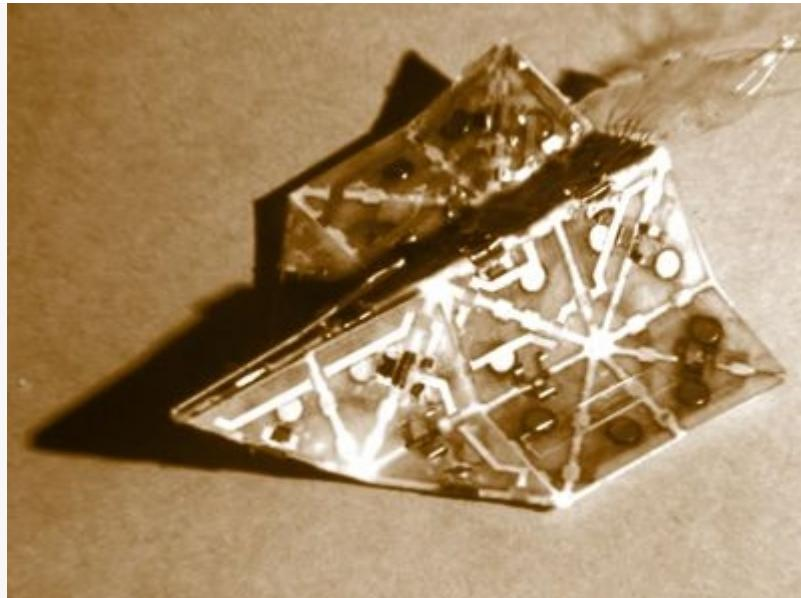
Studded with magnets and electronic muscles known as actuators, a prototype robot developed at MIT can automatically fold itself into an airplane or an origami boat.
